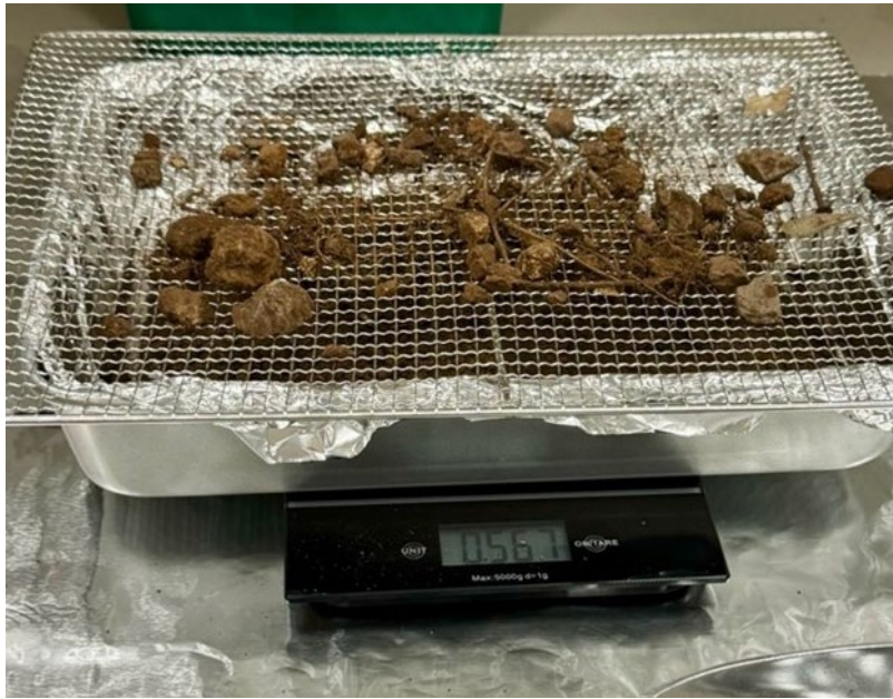
Sieving of composite using .025-inch mesh screen
