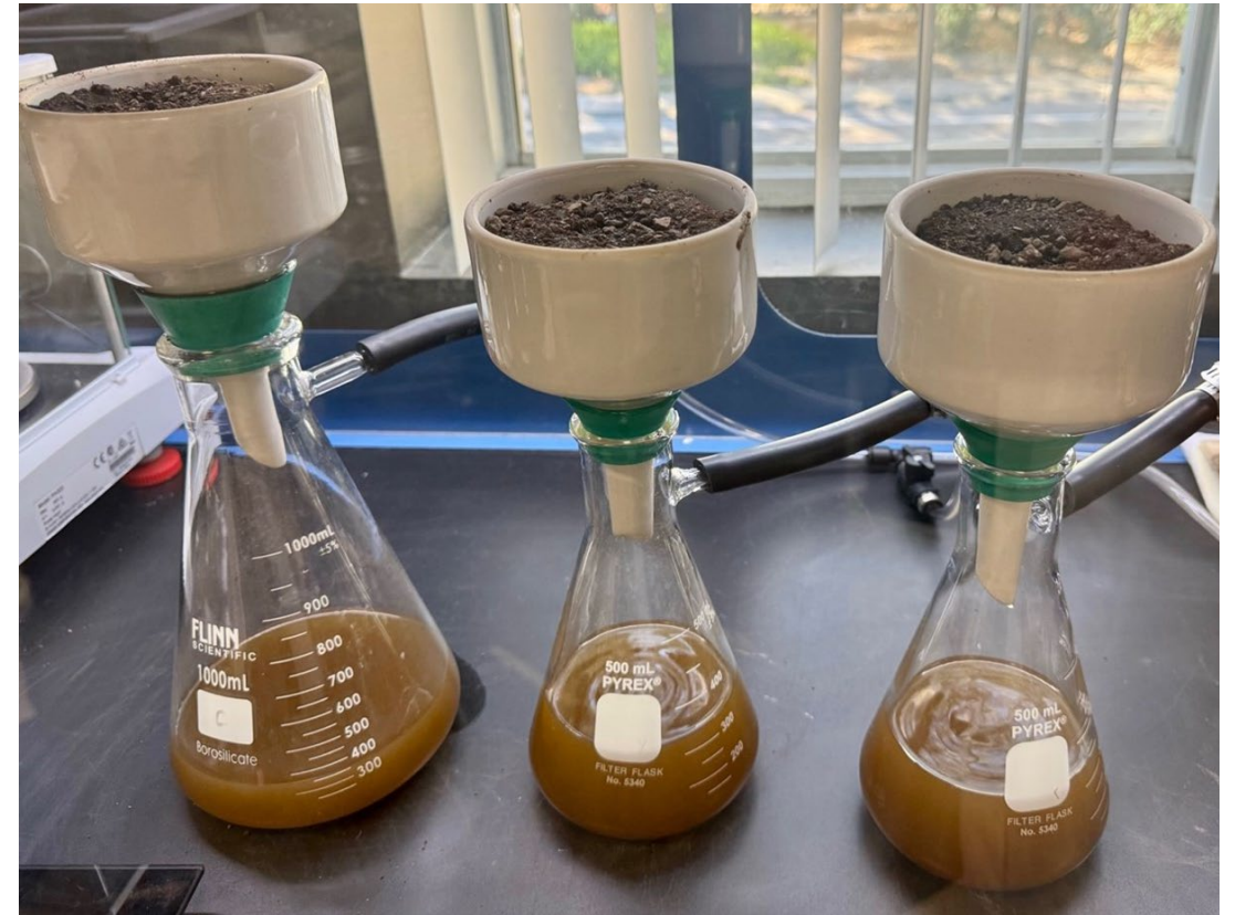
Vacuum filtration to extract reagent
