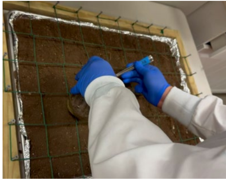
Sampling of composite using multi-incremental sampling
